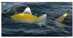
**Fig. 3.** Current ideas on (bio)sensor embodiments for monitoring purposes. (A) *BRAAVOO* automated sampling and readout system for bioluminescence from bacterial bioreporter chips to be embedded on a marine buoy [ref (BIOLUM)]. (B) *Envirobot*, an aquatic robot with multiple sensor segments designed for source tracking and sampling missions [ref (Nano-Tera)]. (C) *SHOAL*, a marine robofish equipped with physical and chemical sensors that may be deployed in swarms [ref (SHOAL)].
