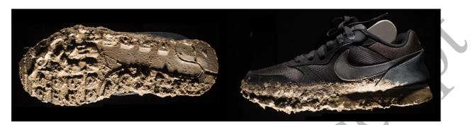
Figure 6. Soil uptake on the sole and the side of a medium profile shoes (Nike Air, size 40, 62 kg), mix soil type, 40% humidity.
