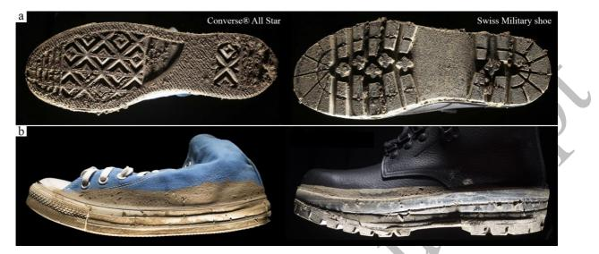
Figure 7. Soil uptake on the sole (a) and the side (b) of a low profile shoe (Converse All Star) and on a high profile shoes (Military shoe), left shoes, soil type 1, 20 % (a) and 55 % (b) humidity.
