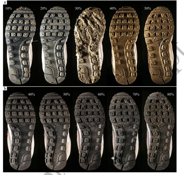
Figure 5. Quantity of soil transferred on Nike Air shoes (size Euro 38) for soil 1 (a) and soil 2 (b) depending on the humidity. Maximum soil transfer was reached at 30 % (a) and 60 % (b) humidity.
