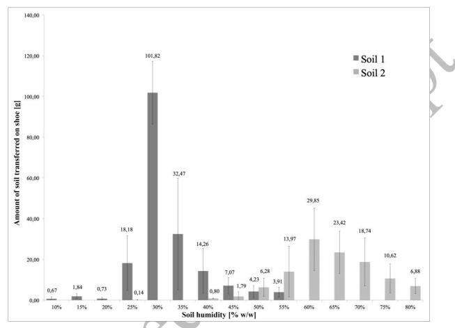
Figure 4. Quantity of soil transferred on Nike Air shoes (size Euro 38) for soil 1 and 2, standard deviations of the 3 experiments are indicated as error bars.
