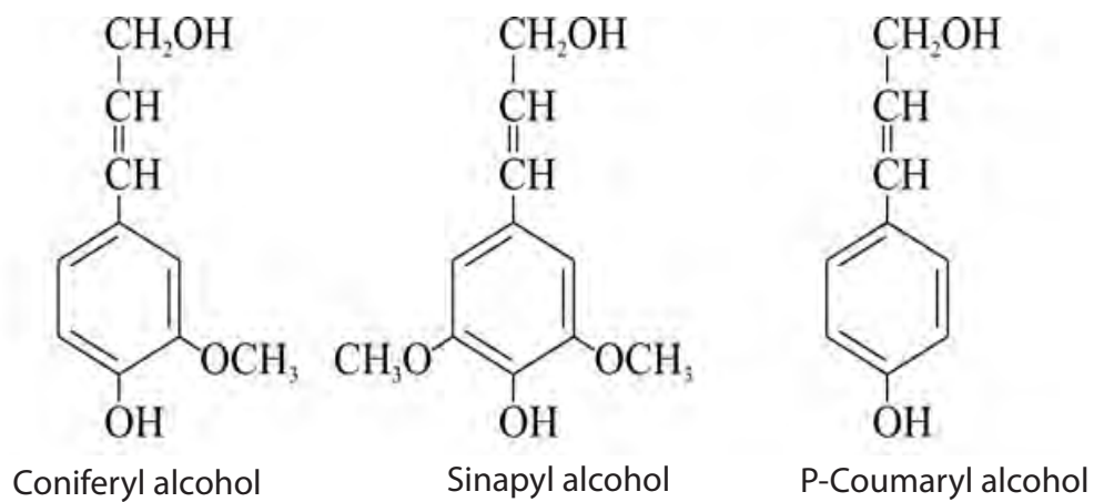
Figure 5: Structure of the three lignin monomers (monolignols).
