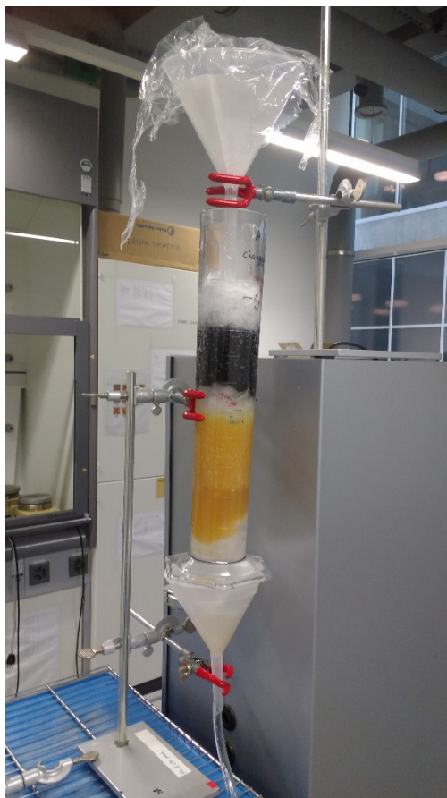
Appendix Fig. 8.18. Sodium polytungstate rinsing column.
