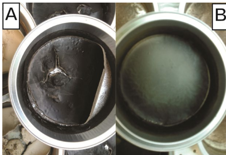
Appendix Fig. 8.16. Density fractionation pre-testing revealed a glass bead was necessary to ensure that the heavy fraction (HF) were thoroughly rinsed. A) This sample was not agitated with a glass bead (1 mm) and could not be rinsed properly. The HF aggregated and created a ball that still contained sodium polytungstate (SPT). B) This sample was agitated with a glass bead during the rinsing process and the HF was rinsed homogeneously, removing all SPT.
