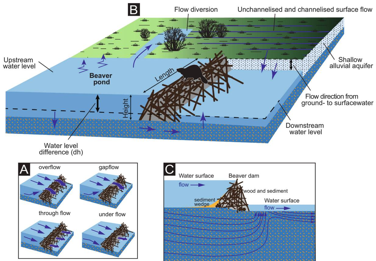
**Fig. 4.** Conceptual models of the influence of beaver dams on surface and subsurface hydrology. Inset A) specifies different types of beaver dams and through flow, modified from Woo and Waddington, 1990. B) Conceptualization of hydrological feedbacks as a result of beaver dam construction on surface and groundwater flow paths and storages. Inset C) illustrates potential hyporheic exchange pathways, modified from White, 1990.
