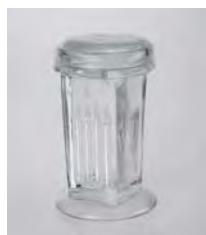
Figure 1: Coplin Jar. In the laboratory, we have jars accommodating 8 and 12 slides.
