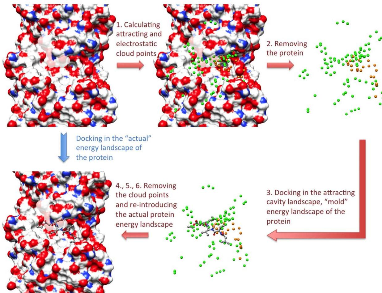
**Figure 1.** AC algorithm. The attracting and electrostatic cloud points are shown as green and orange spheres, respectively. The numbering of the arrows corresponds to the description of the algorithm given in the text.
