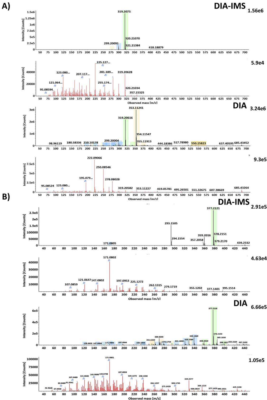
**Fig. 2.** Comparison of HRMS MS spectra (in black) and MS/MS spectra (in red) of (A) flucortolone measured in standard sample and (B) fluoxymesterone metabolite M2 measured in urine sample. (For interpretation of the references to colour in this figure legend, the reader is referred to the Web version of this article.)
