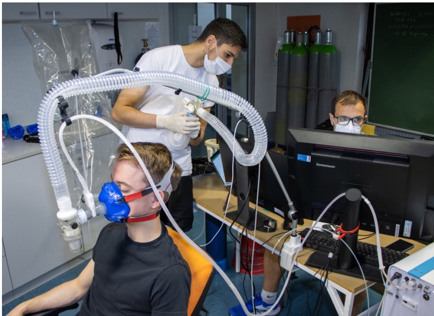
Figure 37. Experimental setup of the pure nitrogen breathing test used to assess hypoxic chemosensitivity in our participants. In the back of the picture, a plastic bag filled with 100% nitrogen was connected via a three-way valve to the mask of the participants. Pulmonary ventilation and peripheral oxygen saturation on the earlobe were continuously measured throughout the test.
