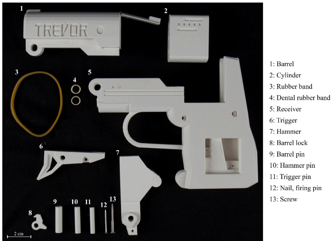
Fig. A3. Disassembled TREVOR. Parts 3 and 4 (different rubber bands), 12 (firing pin) and 13 (screw) are not 3D-printed.
