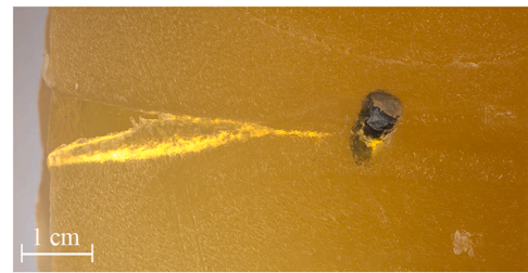
Fig. 6. Cavity in the ballistic soap (side view) and projectile's backwards spin; the bullet was fired with the Songbird in .22 Long Rifle caliber.
