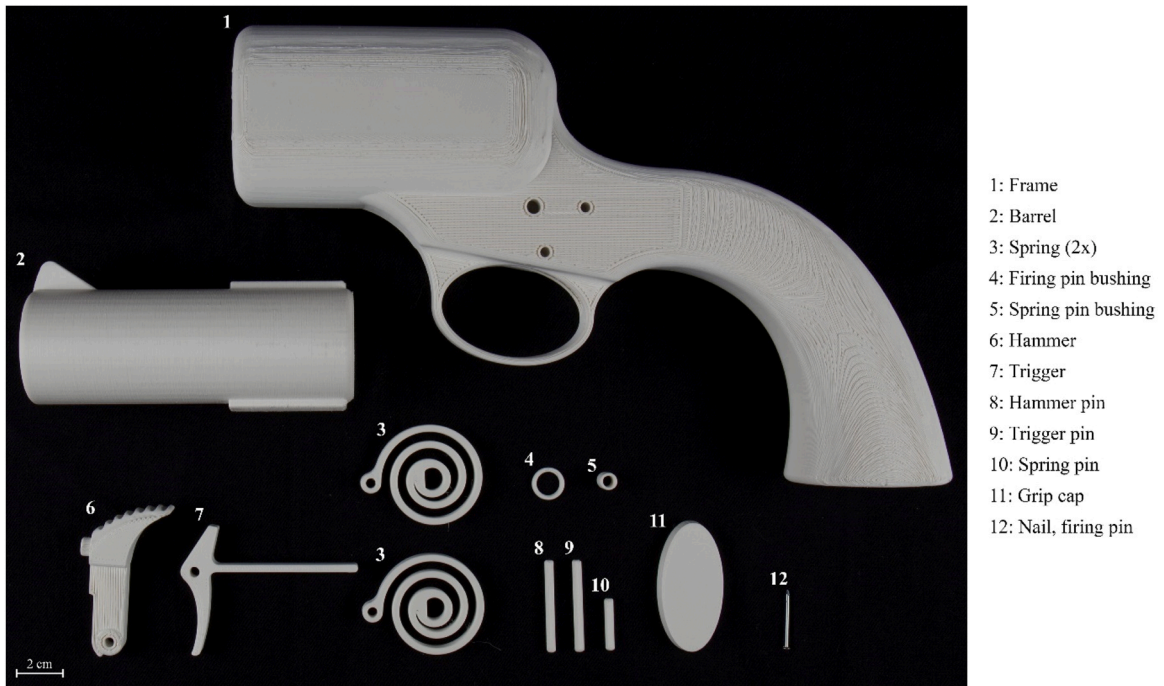
Fig. A4. Disassembled Grizzly. Part 12 (firing pin) is not 3D-printed.
