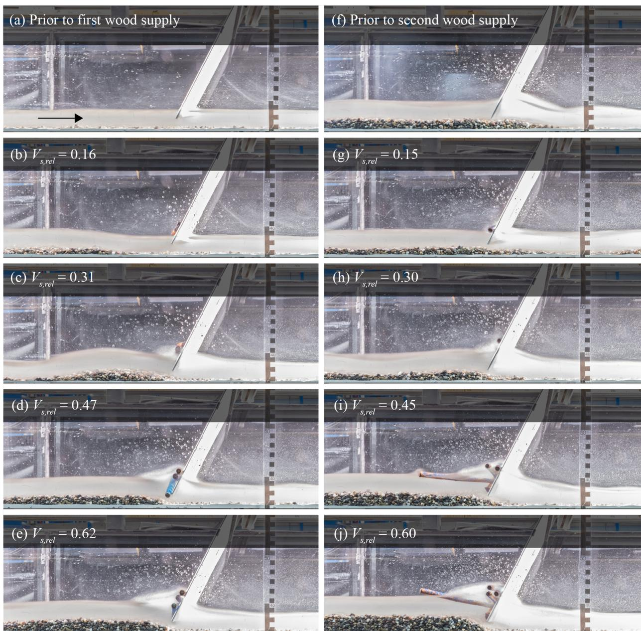
**Figure 12.** LW accumulation and bedload deposition at the inclined bar screen for test V15 with increasing  $V_{s,rel}$ . Panels (a–e) illustrate first run and panels (f–j) second run. (a) Prior to first wood supply, (b)  $V_{s,rel} = 0.16$ , (c)  $V_{s,rel} = 0.31$ , (d)  $V_{s,rel} = 0.47$ , (e)  $V_{s,rel} = 0.62$ , (f) after wood removal of first run and prior to second wood supply, (g)  $V_{s,rel} = 0.15$ , (h)  $V_{s,rel} = 0.30$ , (i)  $V_{s,rel} = 0.45$ , (j)  $V_{s,rel} = 0.60$ .
