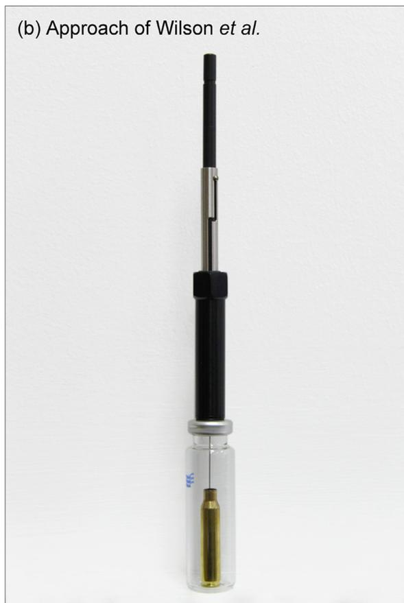
**Fig. 4.** Sampling of a 5.56 mm NATO spent casing using SPME, as suggested by (a) Andrasko *et al.* [34] (using a cork to stop the opening) and (b) Wilson *et al.* [55] (through putting the shell/cartridge in a vial).
