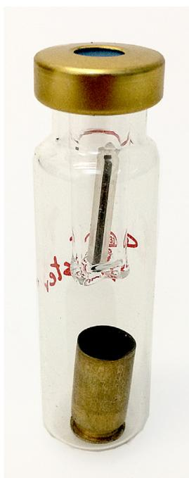
**Fig. 5.** Sampling of cartridges using HSSE, as suggested by Gallidabino *et al.* [64]. The HSSE extraction bar is put in a special insert in the extraction vial, just above the cartridge to analyse.
