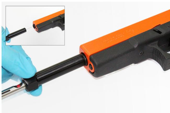
**Fig. 3.** Sampling of a 9mm Parabellum pistol from the muzzle using SPME, as suggested by Andrasko *et al.* [34].
