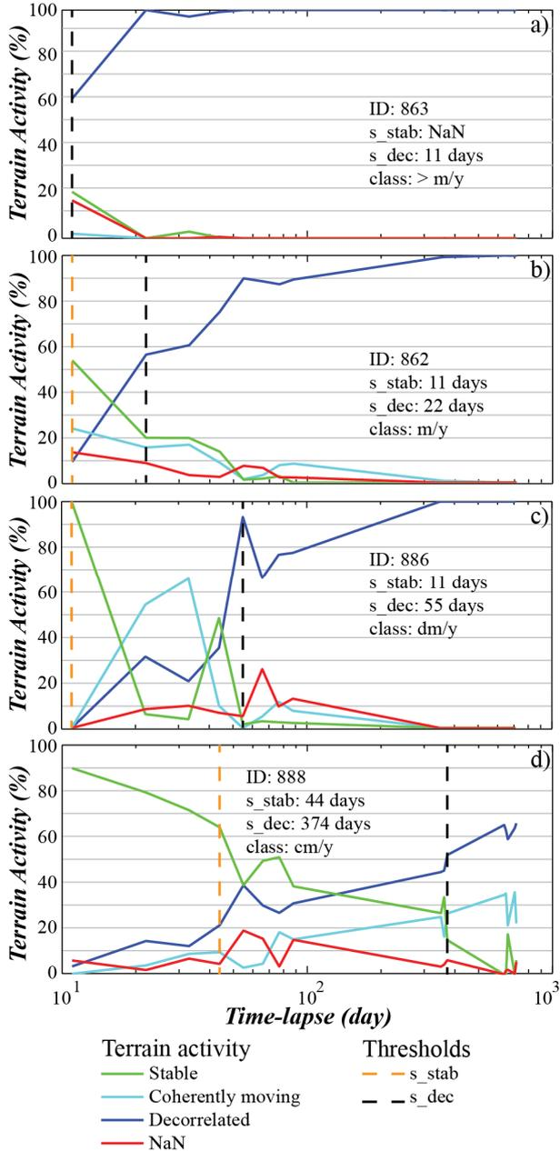
Figure 3: Terrain activities of selected InSAR polygons moving at the velocity rate of a) >m/y, b) m/y, c) dm/y and d) cm/y
