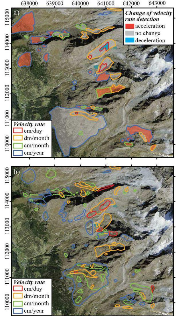
Figure 4. InSAR polygons of the studied area. a) Past InSAR polygons inventory and result of semi-automated change in velocity detection. b) Manual upgrade of InSAR polygons.
