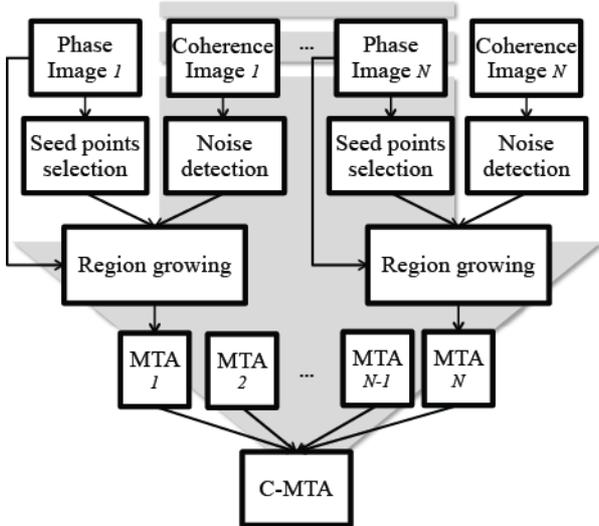
Figure 1: From interferometric phase and coherence images to Combined-Map of Terrain Activity (C-MTA). Process applied to a selected set of  $N$  interferograms having the same time-lapse.
