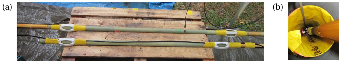
Figure 1.12 – (a) Image of the 100 MHz MALÅ GPR receiver and transmitter antennas used for data acquisition, fitted with custom-made centralizers (white). (b) Image of the transmitter antenna in the GPR monitoring borehole that was fitted with a flexible liner (yellow).
