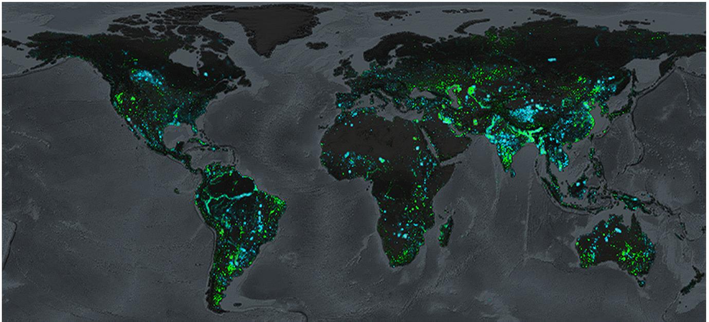
**Figure 5** | Long-term surface water changes (1985–2016) derived from NASA/USGS Landsat missions (Donchyts *et al.* 2016). The colours depict transitions from water to land (light green) and land to water (blue). Satellite imagery was processed in the Google Earth Engine parallel processing environment.
