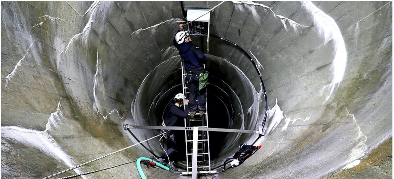
**Figure 2** | Setup of instrumentation for a full-scale measurement campaign in the tunnel spillway of Luzzone dam (Switzerland), where flow velocities of 30 to 40 m/s were sampled (courtesy of VAW, ETH Zurich).
