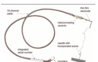
Figure 1. TIME-4H electrode and components. Assembled TIME-4H electrode system with helical cable, polyimide electrode with needle, and Omnetics connector.
