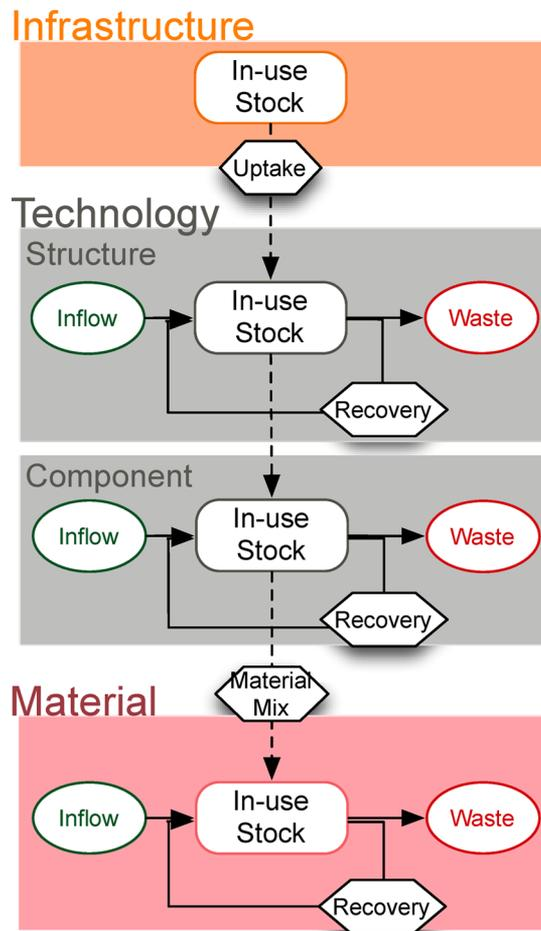
**Figure 1.** Elements of the hierarchical Stocks and Flows Model, from infrastructure stocks to technological structures and components and their material requirements, each resulting in in- and outflows.
