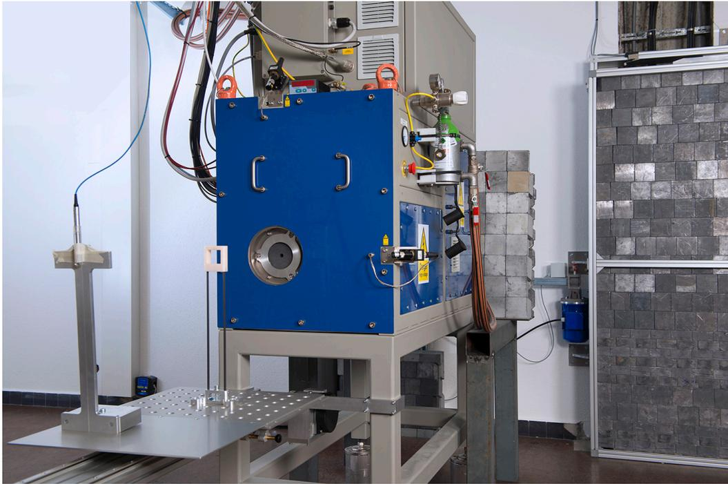
**Figure 4:** Photograph of the eRT6 Oriatron LINAC installed at the CHUV, Lausanne, Switzerland. This LINAC prototype delivers a pulsed electron beam at conventional or ultra-high (FLASH) dose-rates.
