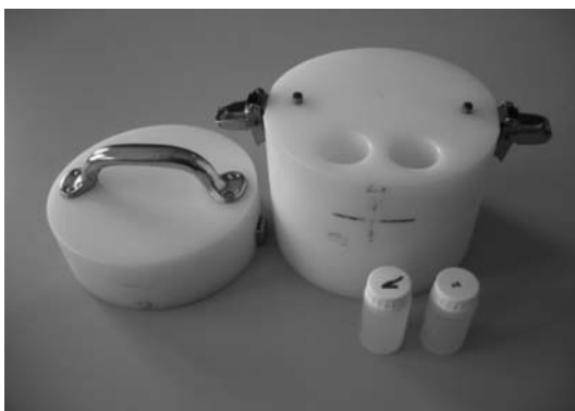
Figure 1. Polyethylene neck phantom bored with two holes for 20 ml radioactive vials.
