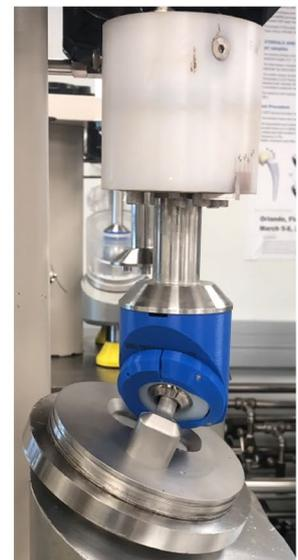
**Fig. 4** (A) Hip simulator mounting with the ADM® dual mobility cup (Stryker, Mahwah, NJ) and custom-made machined cylindrical femoral neck construct for mobile impingement testing. (B) Hip
