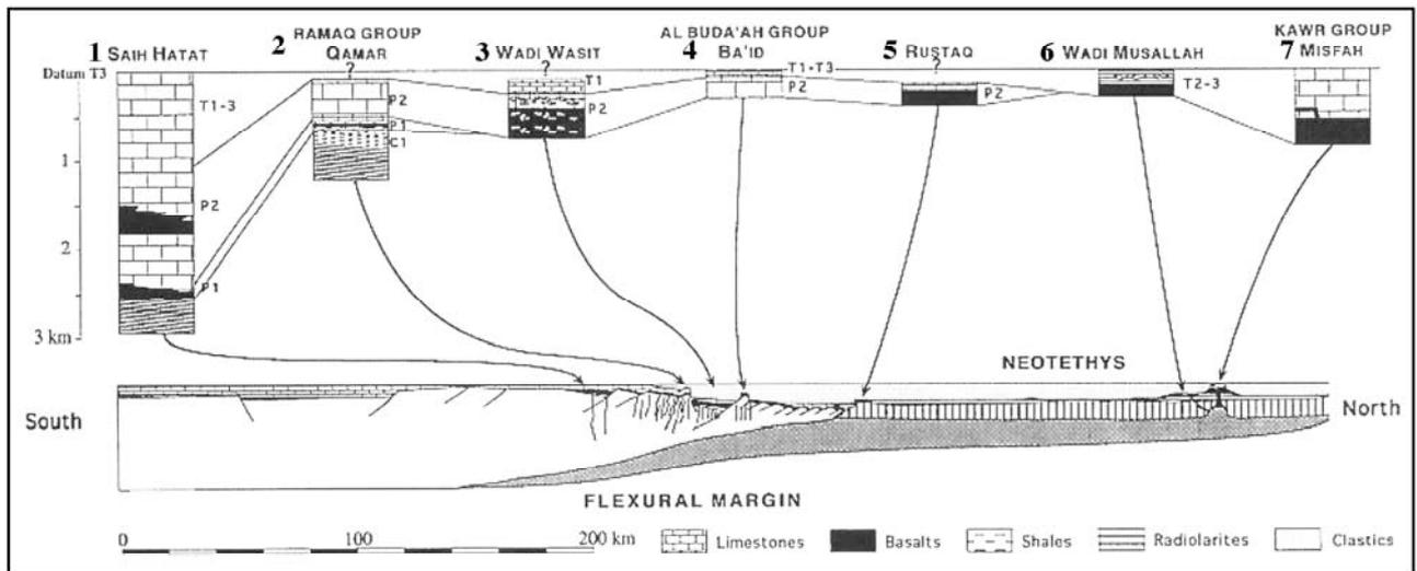
**Fig. 6 -Oman margin in the late Triassic, from proximal (1) to distal (7) (after Pillevuit et al., 1997).**
