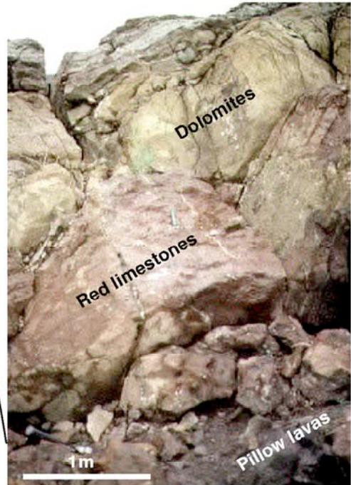
Figure 15- The Rustaq section 1 outcrop.. Details of the sedimentary cover above the pillow lavas.
