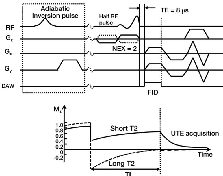
**Figure 3:** IR UTE sequence. An adiabatic IR pulse was used to invert and null the relatively longer T2 signal from meniscal tissues and fat, while leaving the shorter T2 calcification largely unaffected. The inversion time (110 msec) was chosen near the null point of the longer T2 components. DAW = data acquisition window; FID = free induction decay;  $G_z, G_x, G_y$  = gradients in z, x, and y axes, respectively; NEX = number of signals acquired; RF = radiofrequency; TE = echo time.
