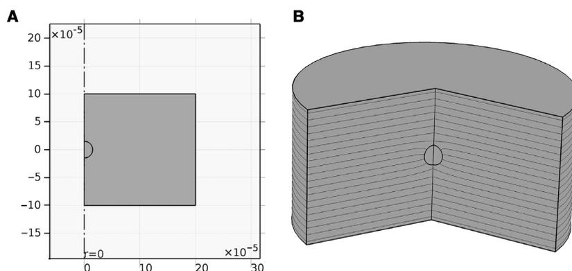
**Figure 3.** (A) 2D axisymmetry model for a single spherical cell between two plate electrodes. The dashed-dot line shows the symmetry axis. The upper and lower electrodes are shown by arrows in the figure. (B) A section of the 3D view of the model. The lines in the figure show the contours of electric potential. It can be seen that the lines are bent around the cell due to the presence of the cell.
