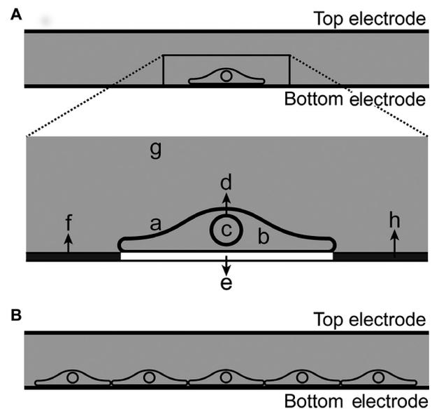
**Figure 2.** (A) Geometry of an attached cell used in the modeling, including cell membrane, a; cytoplasm, b; nucleus, c; nucleus membrane, d; material below the cell, e; material covering the slides around the cell, f; buffer on top of the cell, g; and bottom electrode, h. (B) Geometry of adjacent cells in a multicellular layer.
