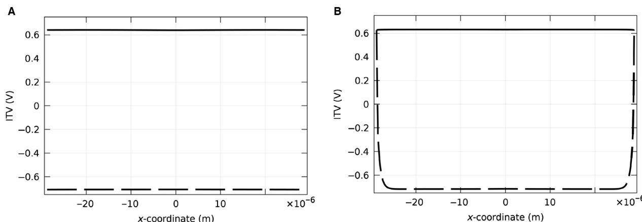
**Figure 5.** ITV in static study for a single cell in (A) a real monolayer of the cells on the substrate and (B) a simplified model replacing all other cells with a layer that has characteristics of the cell membrane. The solid lines show the ITV for the apical side, and the dashed lines indicate ITV for the basal side of the cell. These results show that the actual model of a monolayer and the simplified model are within 95% of each other.
