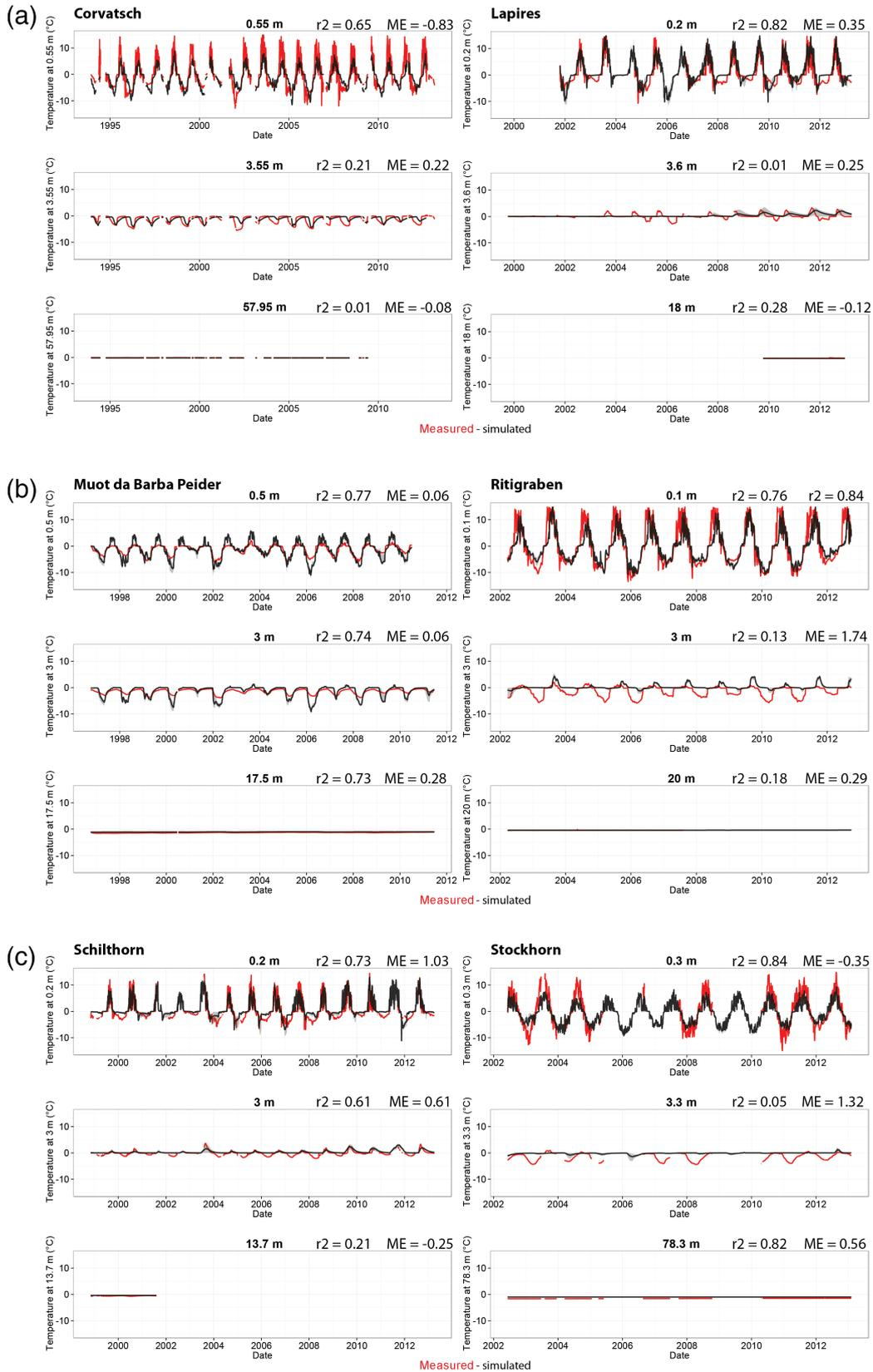
**Figure 6.** (a) Comparison of simulated (black) and measured (red) temperature during the calibration period at six sites at three different depths: one close to the surface, one around 3 m and one close to the lower boundary of the model for Corvatsch and Lapies. (b) As in (a) but for Muot da Barba Peider and Ritigraben. (c) As in (a) but for Schilthorn and Stockhorn.
