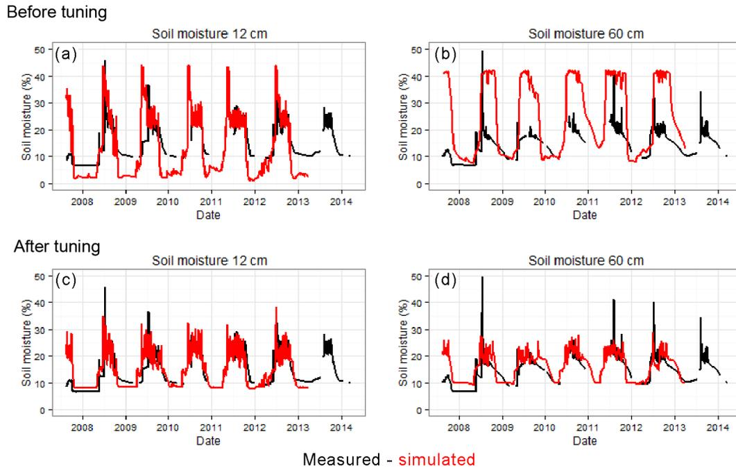
**Figure 9.** Comparison of the simulated (red) and measured (black) soil moisture data at 12 cm (left panels) and 60 cm (right panels) at SCH. Panels (a) and (b) show the results for soil moisture of the best thermal calibration, while (c) and (d) show the results after a further calibration of the soil physical parameter of the water retention curve, showing that the calibration can be further improved with additional data sets.
