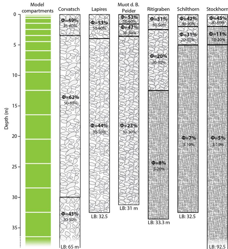
**Figure 3.** Description of the model layers as defined in the model (green) and of the simulated subsurface structure for each site. The depths of the horizons were estimated by experts, based on data from boreholes and geophysical surveys, whereas the porosity  $\Phi$  is defined by the GLUE calibration based on the ranges estimated by the experts (given below the GLUE estimated porosity values). The maximum depth for each site (lower boundary, LB) is given below each column.
