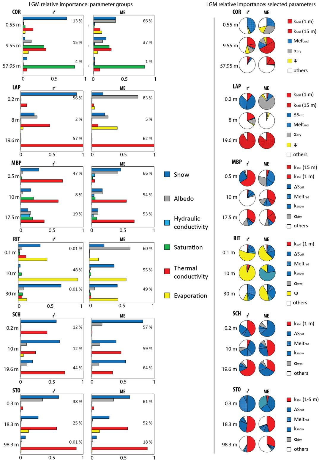
**Figure 5.** Left panel: LGM relative importance of six groups of parameters (snow, albedo, hydraulic conductivity, saturation, thermal conductivity and evaporation) on the  $r^2$  (left row) and the ME (right row) at three different depths. The percentage indicates the total LGM absolute importance. Right panel: LGM relative importance of the most sensitive parameters that were selected for the second step of the calibration procedure.
