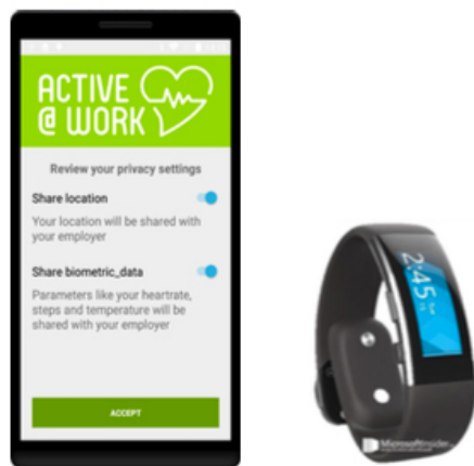
Figure 1. Active@Work mobile app and fitness tracker for collecting physiological data of employees
