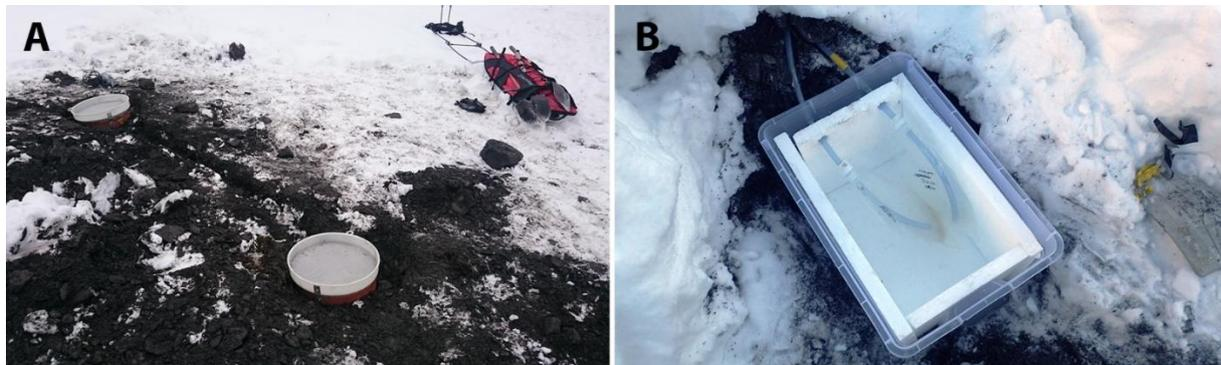
Figure 35. (A) Picture of the co-located lysimeters next to the Chalet weather station. (B) A trench allows a tube to collect independently the melted water from each raingauge in two bags in an insulated plastic box at lower altitude.
