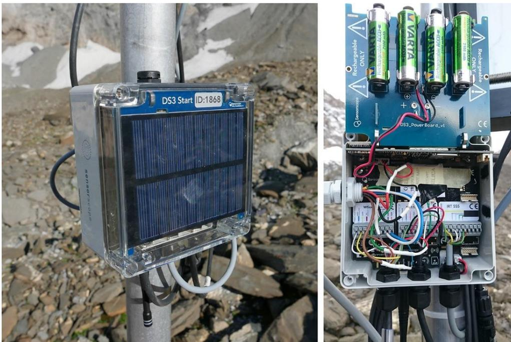
*Figure 19. A Sensorscope datalogger at the Glacier weather station. Each datalogger is energetically self-sufficient, with a solar panel and batteries to supply low consumption sensors up to 5 days without sun. Each box can receive 3 modules, each connected to a sensor. An additional card can transform a datalogger into a master station and transmit the data to a server using the mobile 4G LTE network.*
