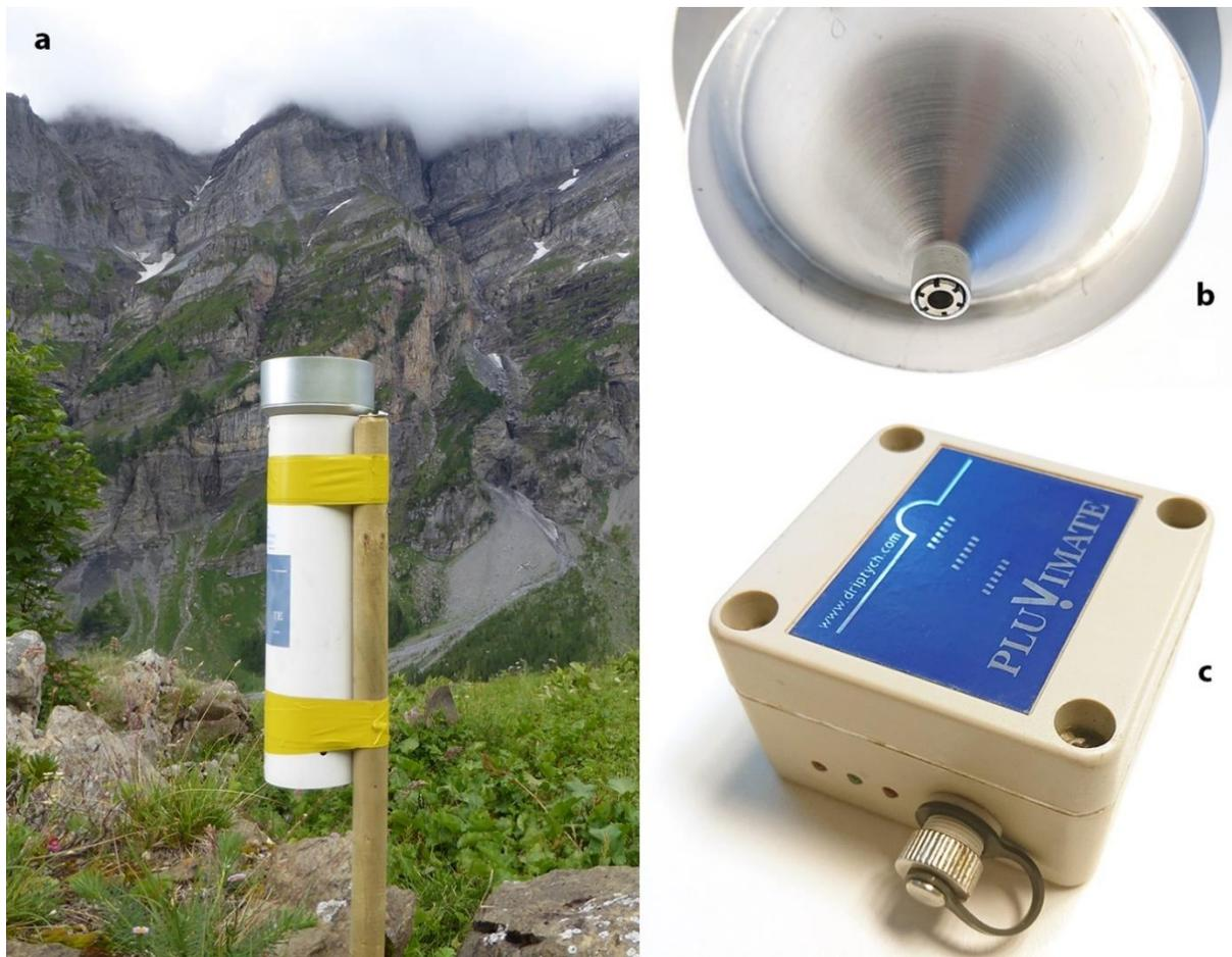
*Figure 31. Drop-counting rain gauge used. The Pluvimate is set-up vertically between 0.8 and 1.2 meters above the ground (a). A tip at the end of the funnel (b) creates a calibrated drop of water that falls on the sensor, (c) which counts and records the number of drops during a given amount of time.*
