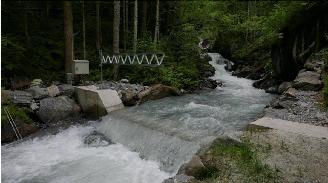
*Figure 8. Trapezoidal shaped weir at the outlet of the Vallon de Nant. The metallic arm holds the optical height gauge device above the middle point of the weir. Temperature, conductivity, and turbidity probes are located downstream within the 2 metal tubes visible on the left. Sediment transport is measured using geophones located under each metal plate across the weir section.*
