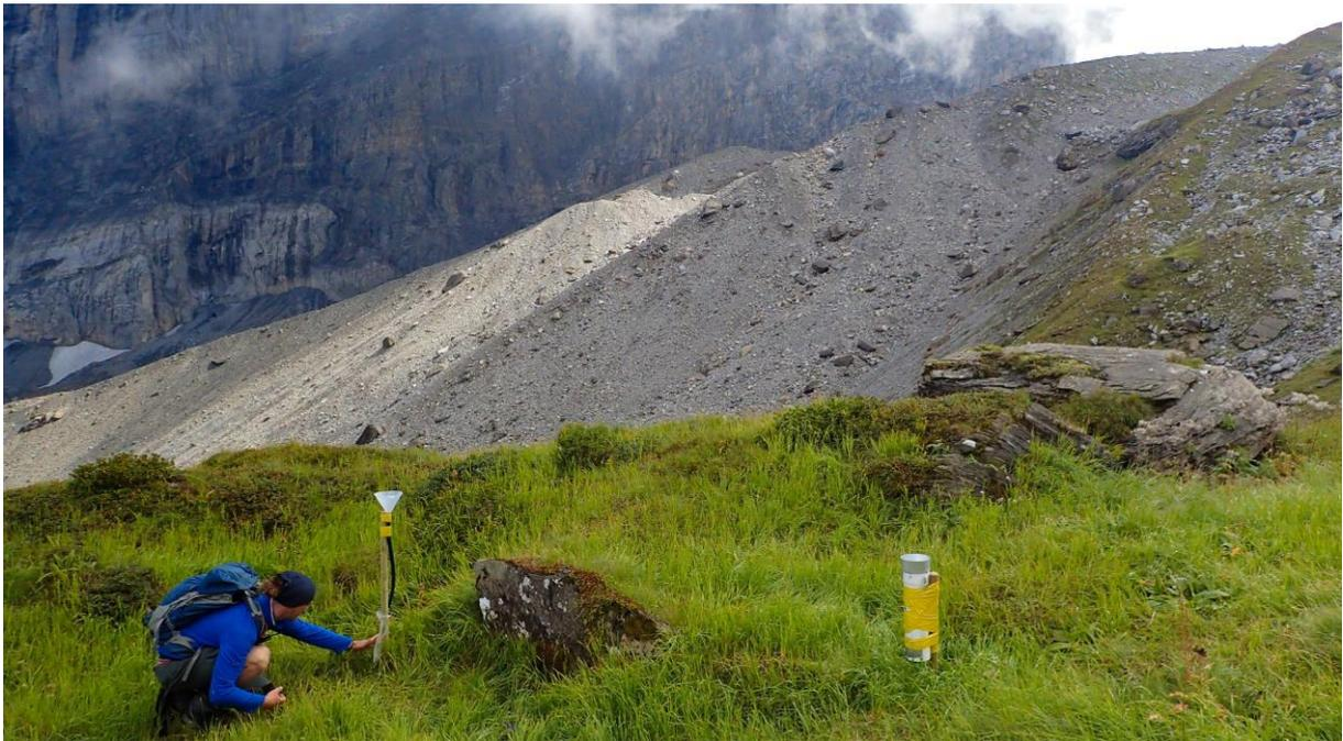
**Photograph:** Rainfall intensity measurement using a Pluvimate (on the right) next to the moraine area.
