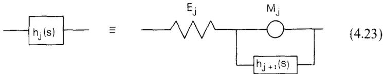
We are then led to the following infinite ladder network representation for the response function:
