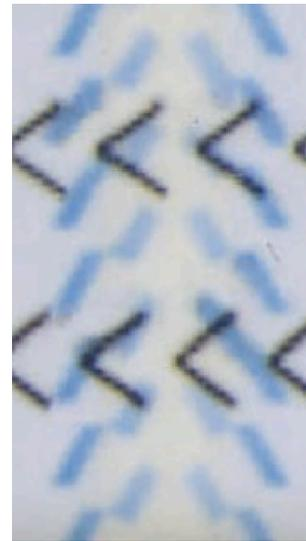
Fig. 13. Discontinuity in the repetitive drawing on a counterfeit Spanish identity card (see the black arrow).
