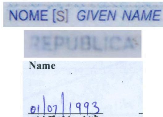
Fig. 15. Defect in the reproduction process: the colour of the 'S' (left) and contrast of the 'R' (right) are not reproduced correctly on a counterfeit Portuguese identity card. Small black spots can be observed on the white background of a counterfeit Eritrean driving licence (bottom).
