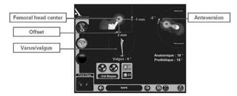
Fig. 8. During the insertion of the rasp, the femoral antetorsion, the lateralization of the femoral center of rotation, the varus/valgus angle, and the height of the center of the prosthetic femoral head are displayed
