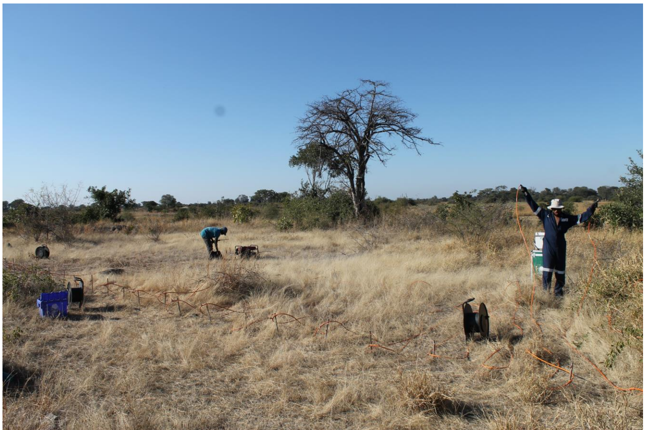
Setting up an ERT survey profile
