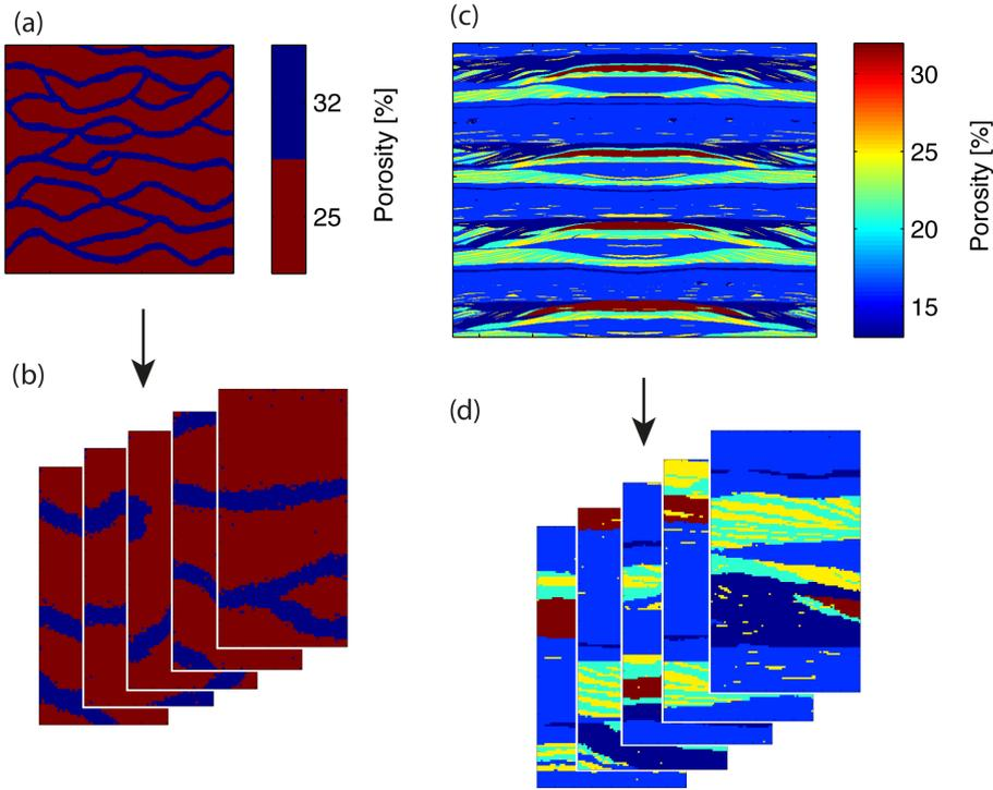
**Figure 3.** Training images for the channels case (a), the fluvial deposits case (c) and multiple-point statistics realizations thereof (b and d). Note that the full ensemble of TI realizations contains 1000 realizations for both cases.
